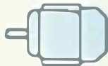
B6 IM 1051 Foot wall mounted with feet on left-hand side when viewed from D.E.
