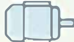
B7 IM 1061 Foot wall mounted with feet on right- hand side when viewed from D.E.
